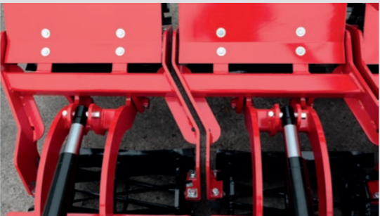
Z-spaced rows avoid gaps between roller sections
