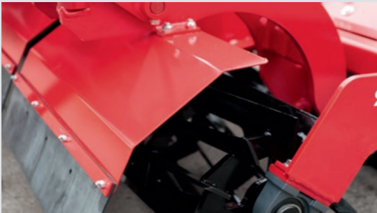
Guard plates protect the tractor from stone damage
