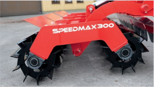
Bogie frame ensures smooth operation even on uneven terrain
