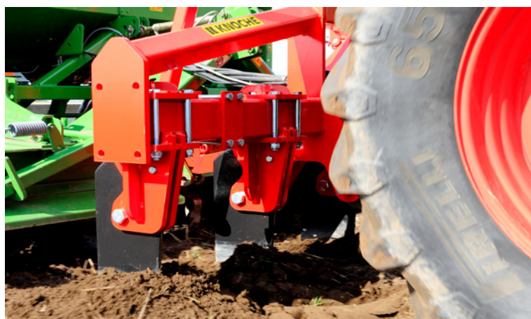
The chisel cultivators' tines ensure deep soil tillage even on hard soils.
