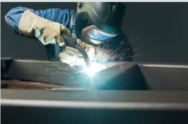
Frame manufacturing with DIN EN ISO 9606-1 certified welding
