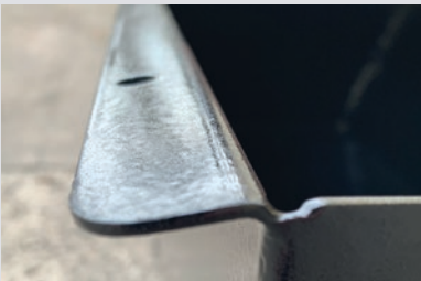
Stone collector made from 2 mm steel
